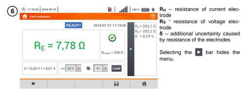
Save the measurement to the meter memory using the 🔲 icon. A detailed description of memory management is contained in section 5.3.
