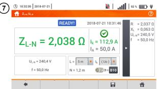
$\begin{aligned} R - \text{resistance of the tested circuit} \\ X_L - \text{reactance of the tested circuit} \\ U_{L\text{-N}} - \text{voltage relative to the neutral conductor} \end{aligned}$
