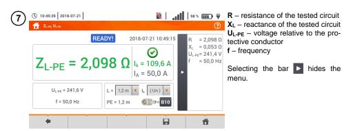
8 Save the measurement to the meter memory using the 🔲 icon. A detailed description of memory management is contained in **section 5.3**.
