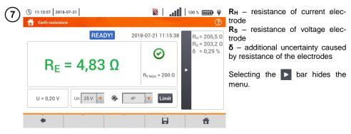
Save the measurement to the meter memory using the licon. A detailed description of memory management is contained in **section 5.3**.
