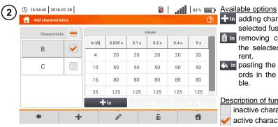
+In adding characteristics for the selected fuse rated current.
