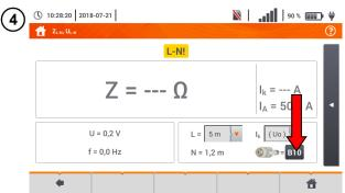
The result can be compared against the acceptable fault loop impedance  $Z_{sdop}$ , determined on the basis of the fuse parameters of the tested circuit:
