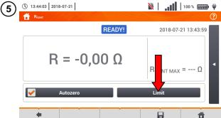
Set the acceptable limit resistance of the measured object.
