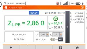
**R** – resistance of the tested circuit X<sub>L</sub> – reactance of the tested circuit UL-PE - voltage relative to the protective conductor
