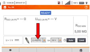
Connect the meter probe or the adapter which the measurements will be performed with.
