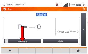
In order to eliminate the impact of the resistance of test leads on measurement result, the compensation (autozeroing) of resistance may be performed. For this purpose, select **Autozero**.
