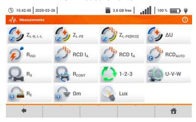
The following tests are available from the **Measurements** menu:
