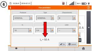
The current is calculated after setting parameters in steps (6)(7).
